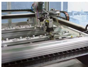
Induction soldering head on servo-controlled axis
